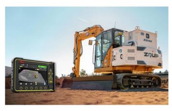
ZQUIP has designed its Modular Power System to deliver reliable, high-performance electric power to heavy machinery. This provides the energy customers need to sustain demanding construction tasks for as long as required. Any construction machine outfitted with the ZQUIP Modular Power System can exchange power modules with any other make or model of ZQUIP machine, ensuring flexibility across various types of heavy equipment.
